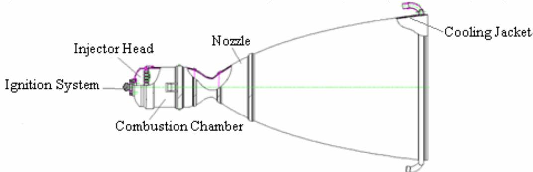
Figure 1: Thrust chamber
