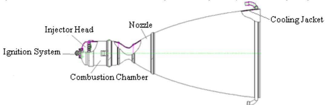
Figure 1: Thrust chamber
