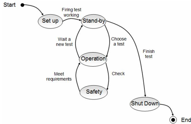
Figure 8: Test Stand State Diagram.
