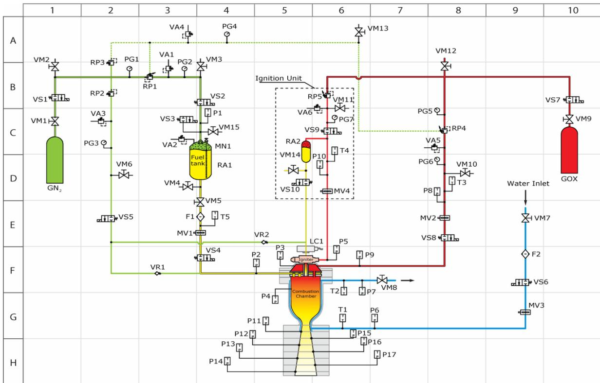
Figure 5: Hydropneumatic scheme.
