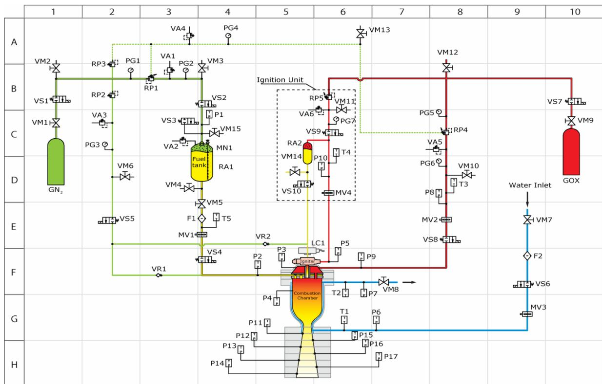
Figure 5: Hydropneumatic scheme.
