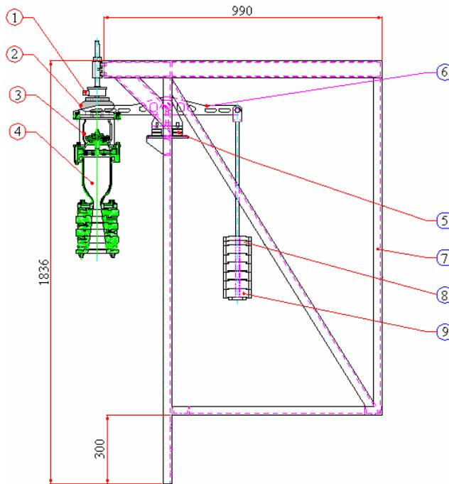
Figure 4: Lateral view of test stand design (engine in longitudinal cut).
