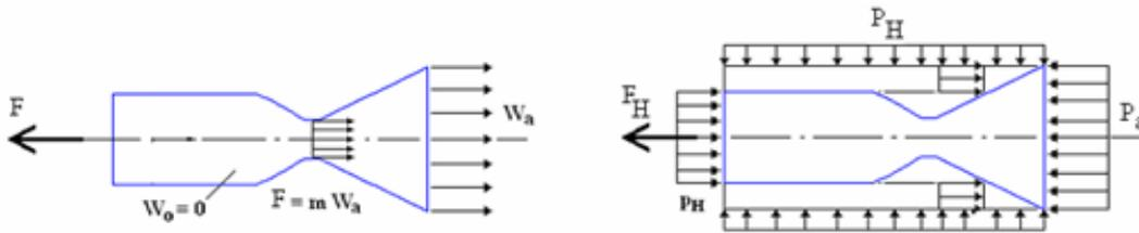
Figure 2: Thrust in the atmospheric conditions.
