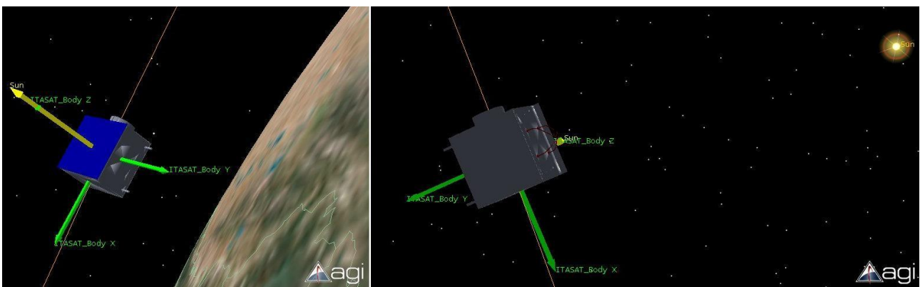
Figure 4. ITASAT sun-aligned body-fixed attitude coordinate frame
