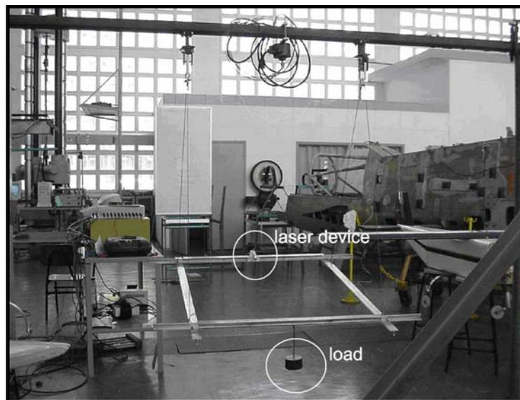
Figure 6 – Swinging gear with laser device and load.
