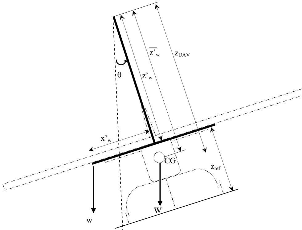
Figure 3 – UAV and swinging gear tilting about x axis.
