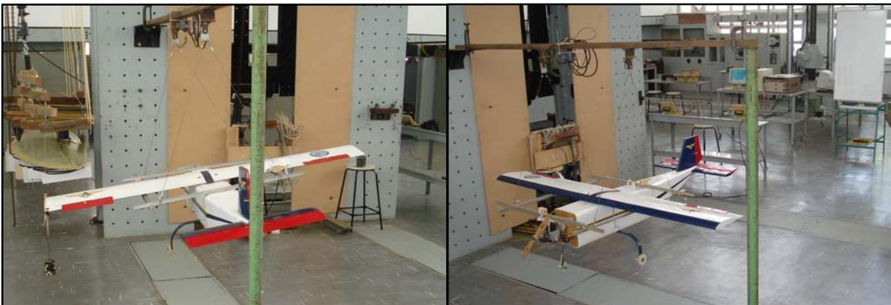
Figure 7 – UAV tilting around x and y axes, respectively.
