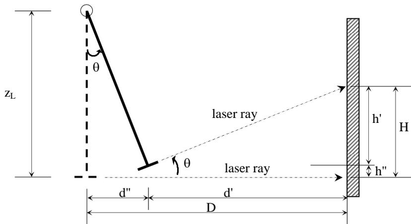
Figure 5 – Experimental determination of tilt angle  $\theta$
