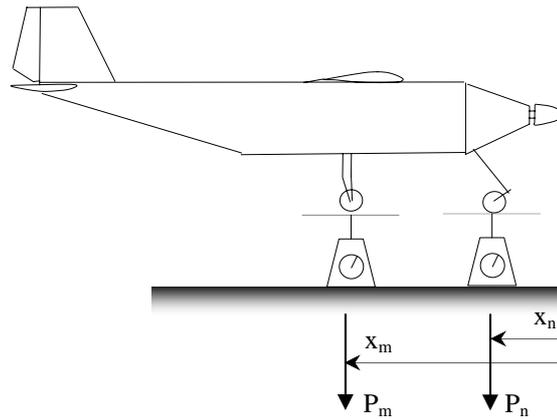
Figure 8 – Determination of x-coordinate of CG
