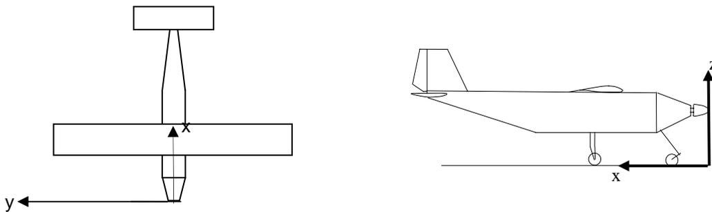
Figure 1 – UAV body axes.
