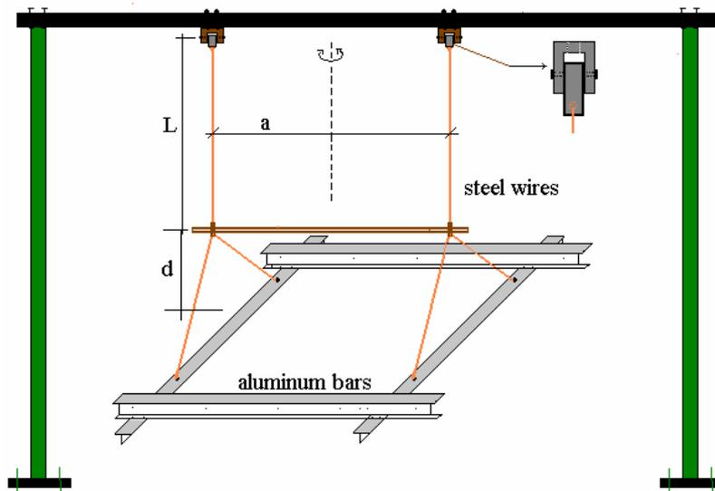
Figure 9 – Bifilar torsion pendulum for determination of  $I_{zz}$
