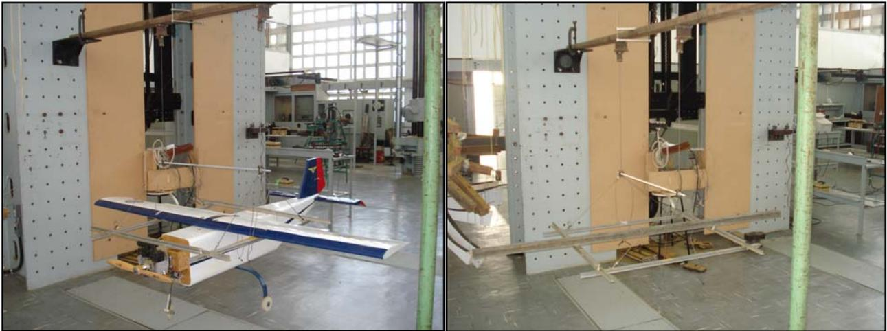
Figure 10 – UAV and bar determination of  $I_{zz}$
