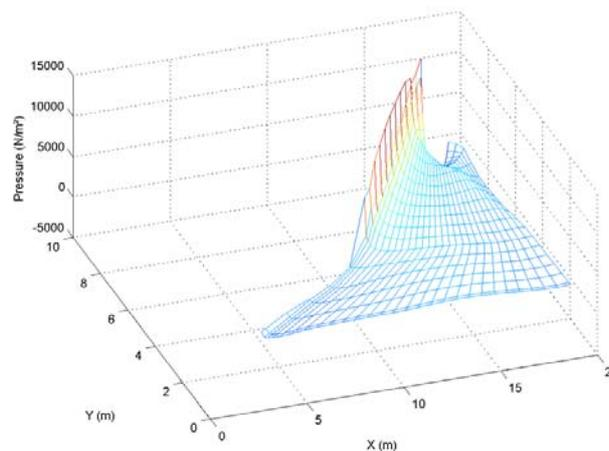
Figure 4: Distribution of the pressure of the aerodynamic on the semi-wing
