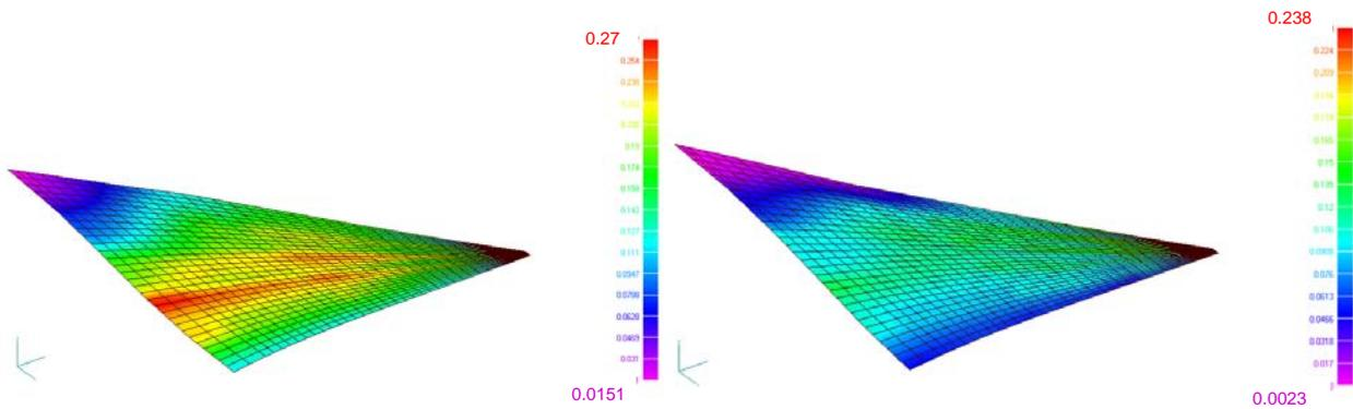
Figure 10: Tsai-Wu criteria for lower (left) and upper skin (right)
