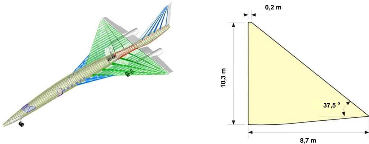
Figure 2: Structural skeleton of the Strider (left) and dimensions of the structure (right).
