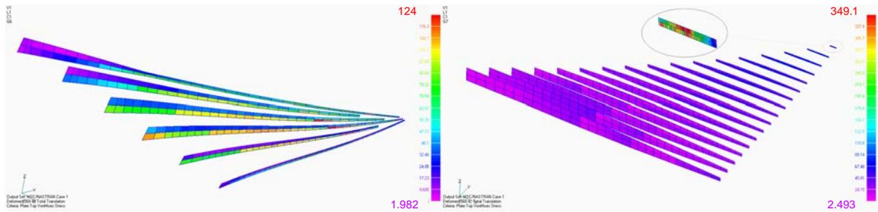
Figure 14: Von Mises tension on the spars (left) and ribs (right)
