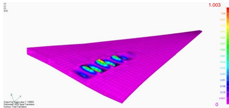
Picture 15: Buckling eigenvalues of the optimized metallic models
