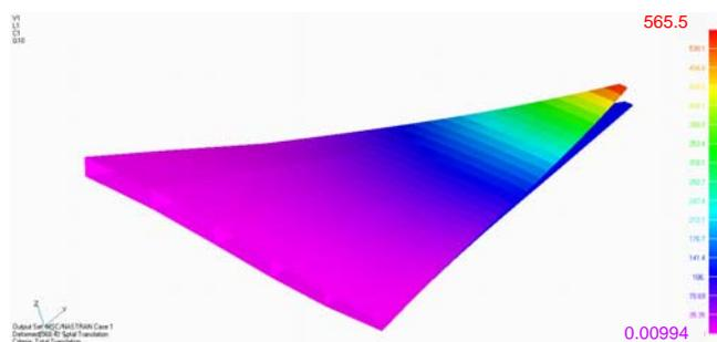
Figure 12: Total deformation of the metallic semi-wing
