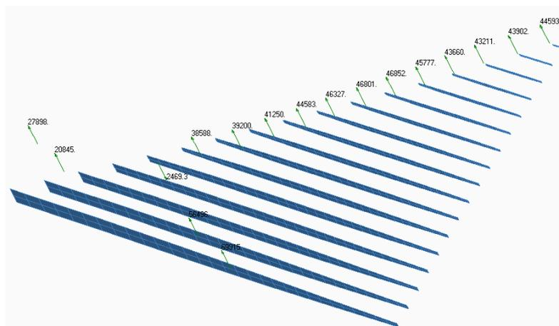
Figure 5: Distribution of effort resulting (N) of the aerodynamic pressure on the rib
