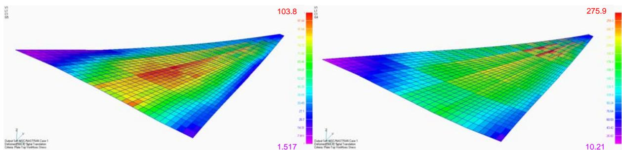
Figure 13: Von Mises tension on the upper (left) and upper skin (right)
