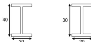
Figure 8: Optimized stringers of upper skin a) root, b) tip (mm)
