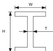
Figure 25: Beam dimensions
