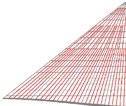
Figure 3: Structural model with spars, ribs and stringers (red)
