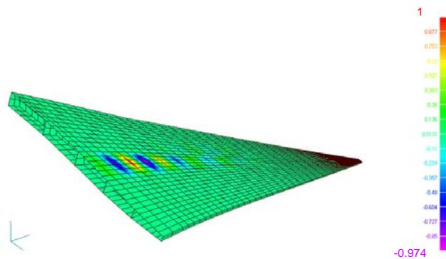
Figure 11: Buckling eigenvalues of the optimized model
