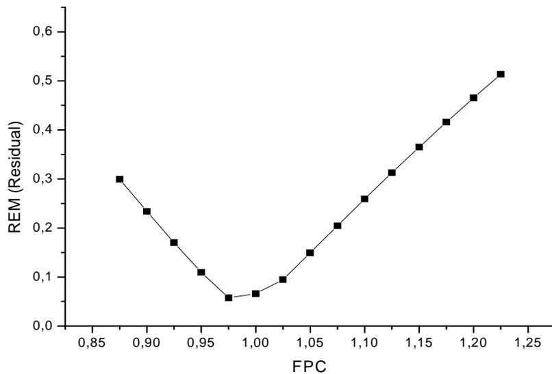
**Figure 1. Minimizing the Residual Error via FPC**
