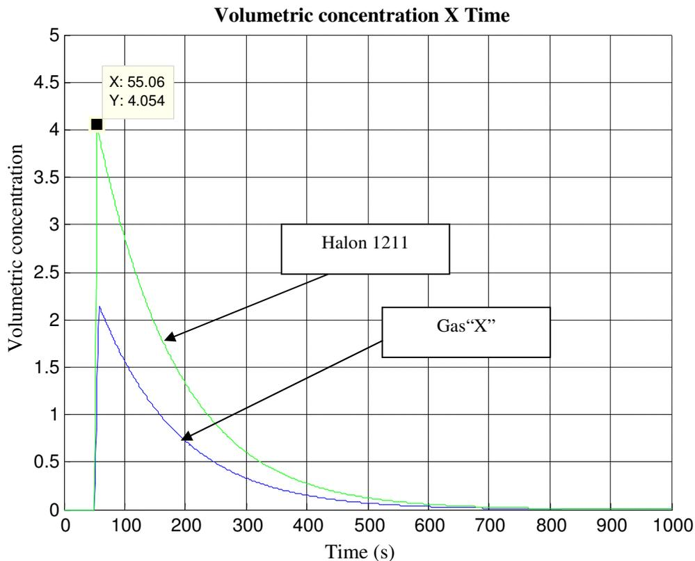
Figure 6 – Volumetric concentration over time for the discharge of Halon and the gas represented by “X”
