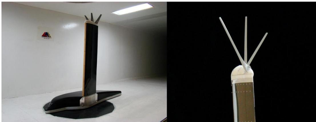
Figure 1: Model prepared for tests, left, and multi-winglets in configuration 1, right
