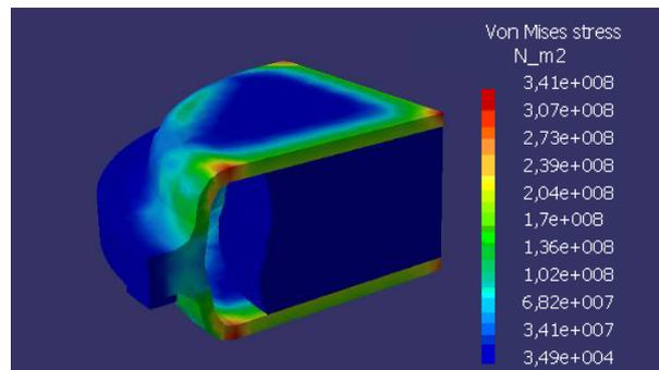
Figure 11. Von Mises stress for shell
