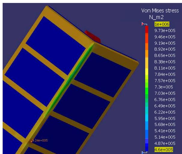
Figure 8. Von Mises stress for elastomeric substrate
