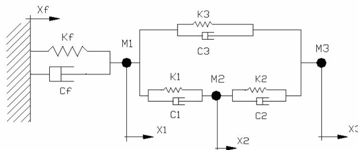
Figure 2. 3 DOF Lumped Parameters model
