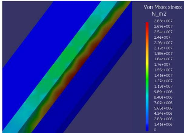
Figure 10. Von Mises stress for shell and rod
