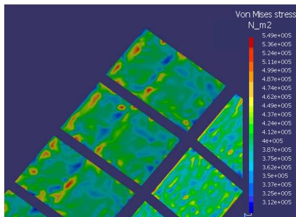
Figure 9. Von Mises stress for solar cells
