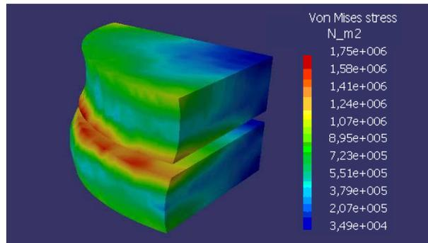
Figure 13. Von Mises stress for elastomer
