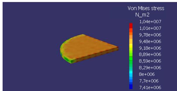
Figure 12. Von Mises stress for electronic PCB
